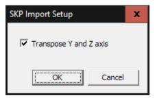
The SketchUp Import Setup dialog includes a Transpose Y and Z option. When checked, this allows SketchUp objects imported into DesignCAD to appear "right side up". This option is provided because DesignCAD uses Y for the vertical axis, whereas SketchUp uses Z for the vertical axis. If this option is left unchecked, SketchUp imports will appear on their sides instead of upright.
