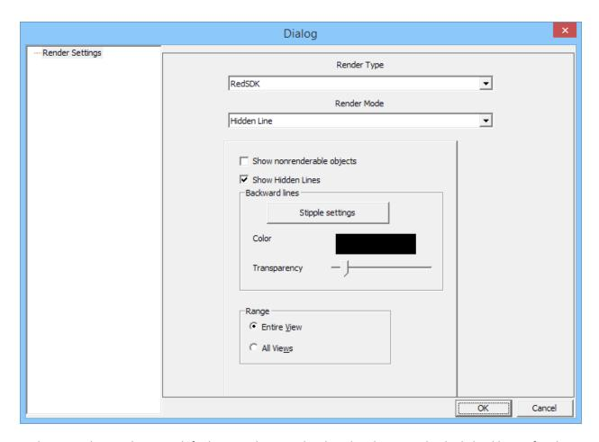
In this case, the Render Type defaults to RedSDK, and rather than having individual checkboxes for showing Text, Dimensions, Lines and Arrows, there's only one checkbox for **Show nonrenderable objects**. Checking or unchecking this box is the same as checking or unchecking all the other types in a GDI or OpenGL view.
